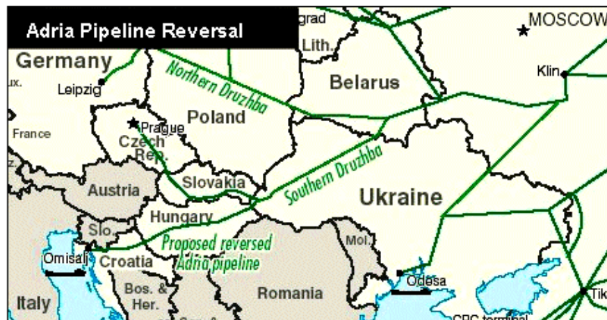
Figure 2. Druzhba and Adria Oil Pipelines
