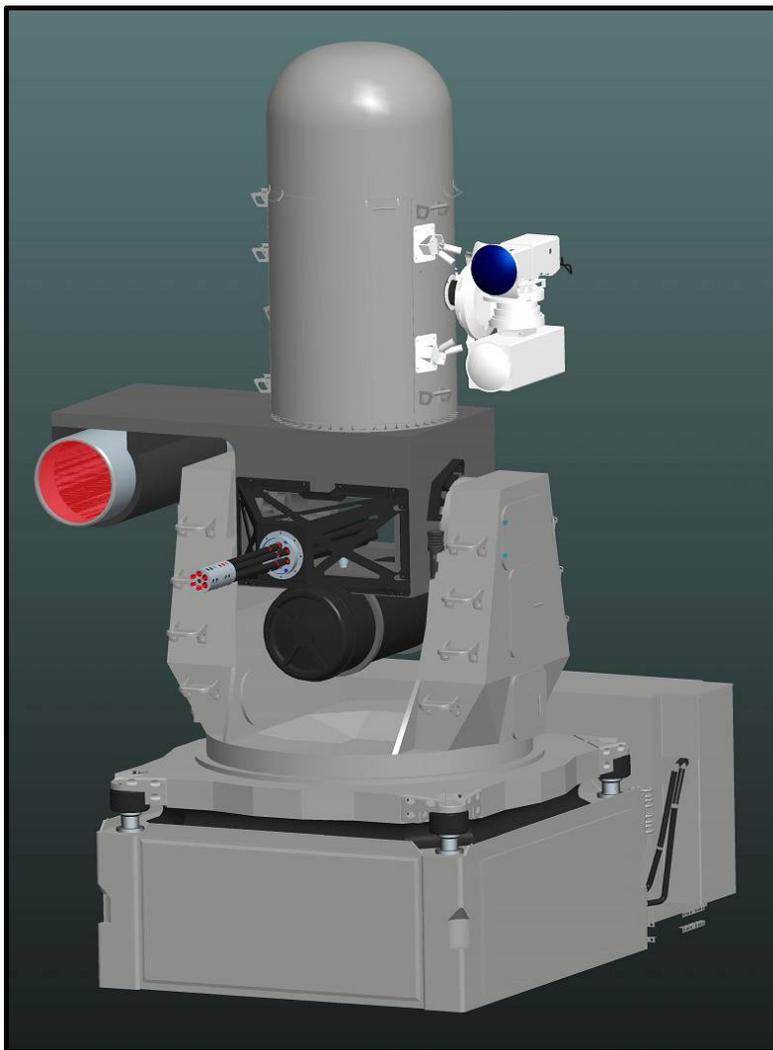
**Source:** Rendering provided by Navy Office of Legislative Affairs, November 3, 2010. In this rendering, the red-colored tube hanging off the left side of the CIWS mount is the LaWS beam director, and the white device bolted to the right side of the CIWS radome is another LaWS component.
