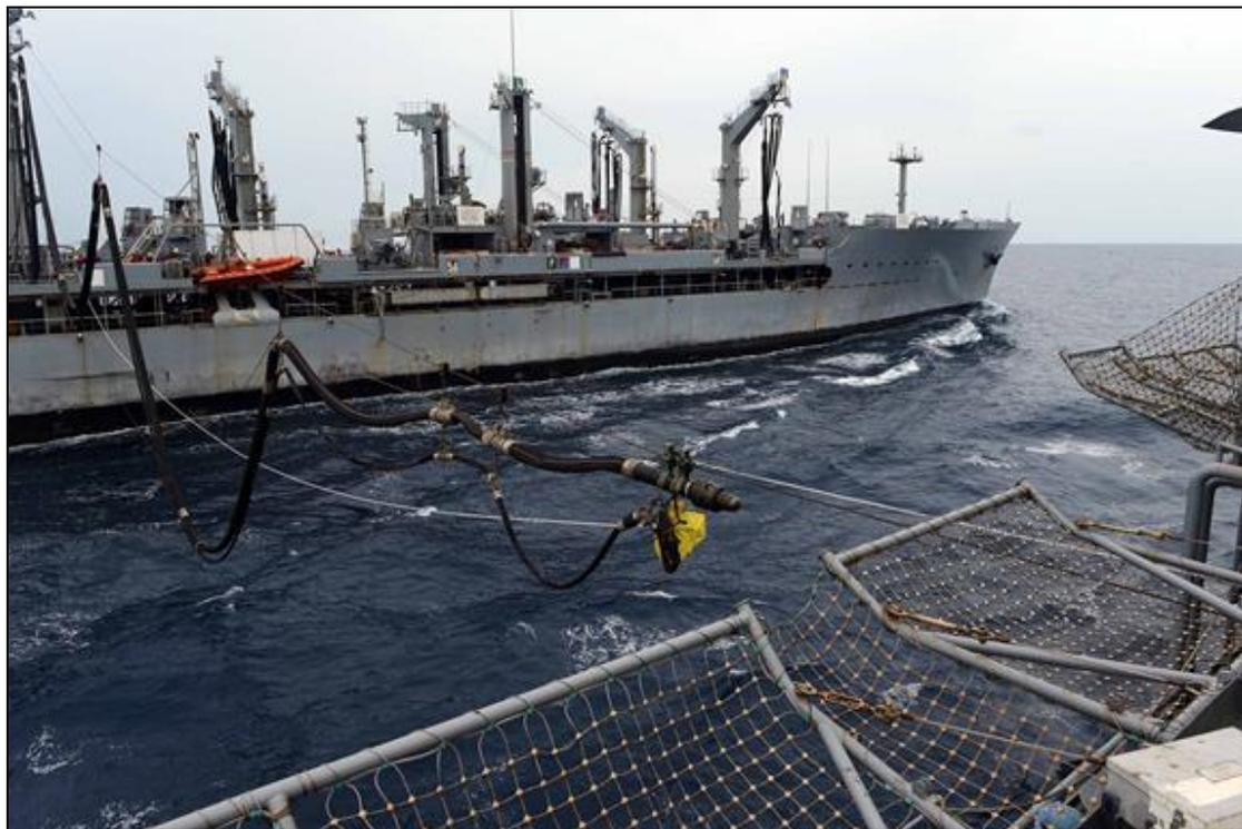
**Source:** Navy photo accessed May 5, 2014, at [http://www.navy.mil/view\\_image.asp?id=163895](http://www.navy.mil/view_image.asp?id=163895). The Navy states that the photo is dated October 24, 2013, and shows the oiler *Tippecanoe* (TAO-199) extending its fuel probe to the Aegis cruiser *USS Antietam* (CG-54), a part of the George Washington (CVN-73) Carrier Strike Group, in the South China Sea.
