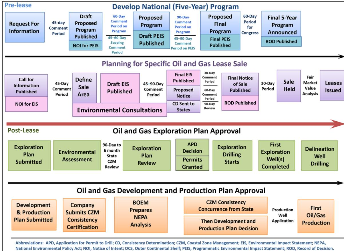
**Source:** BOEM oil and gas leasing flow chart, at <https://www.boem.gov/Oil-and-Gas-Energy-Program/Leasing/Five-Year-Program/BOEM-OCS-Oil-and-Gas-Leasing-Process-Diagram.aspx>.
