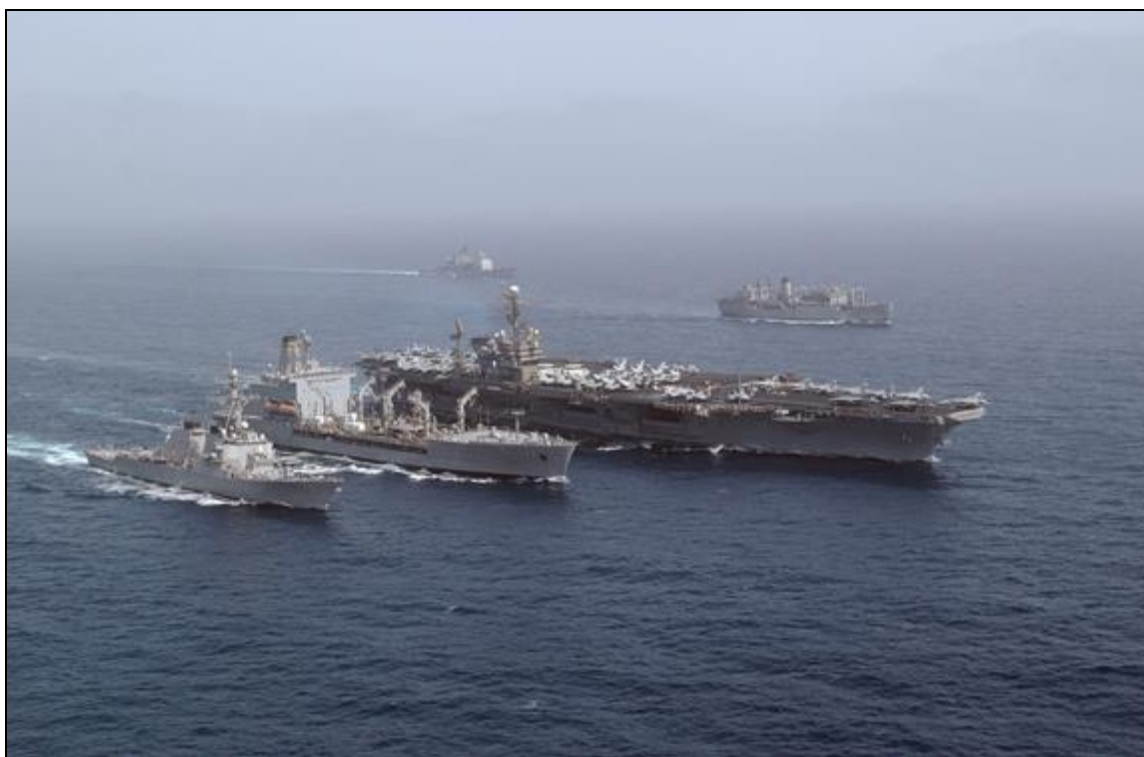
Figure 3. Fleet Oiler Conducting an UNREP
