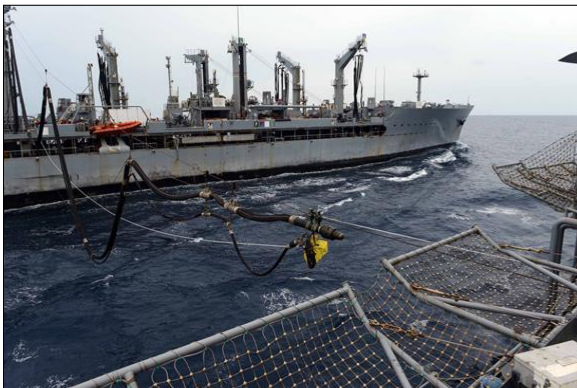
Figure 1. Fleet Oiler Conducting an UNREP
