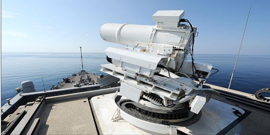
Figure 2. Laser Weapon System (LaWS) on USS Ponce
