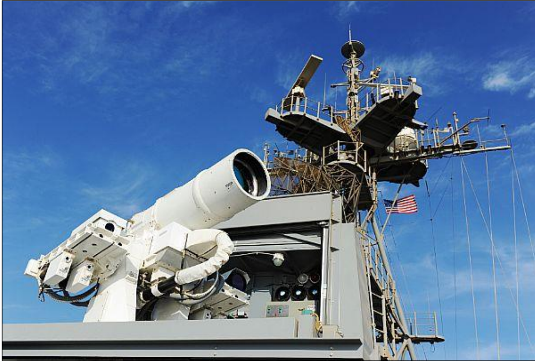
Figure 1. Laser Weapon System (LaWS) on USS Ponce
