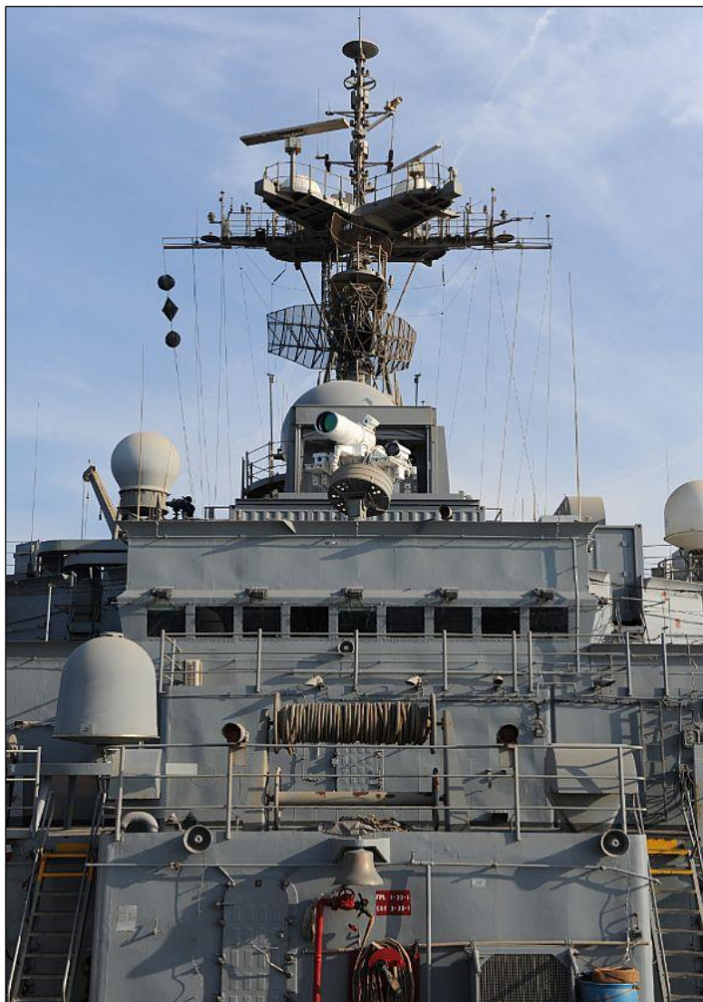
Figure 3. Laser Weapon System (LaWS) on USS Ponce
