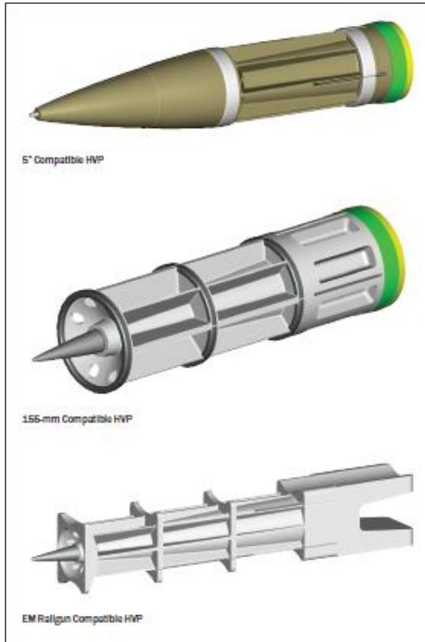
**Source:** BAE Systems, “Hypervelocity Projectile (HVP),” 2014, accessed August 14, 2015, at [http://www.baesystems.com/download/BAES\\_178505/hyper-velocity-projectile—datasheet](http://www.baesystems.com/download/BAES_178505/hyper-velocity-projectile—datasheet).
