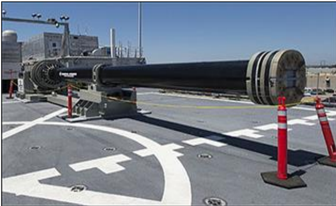
Figure 14. Industry-Built EMRG Prototype Demonstrator General Atomics prototype
